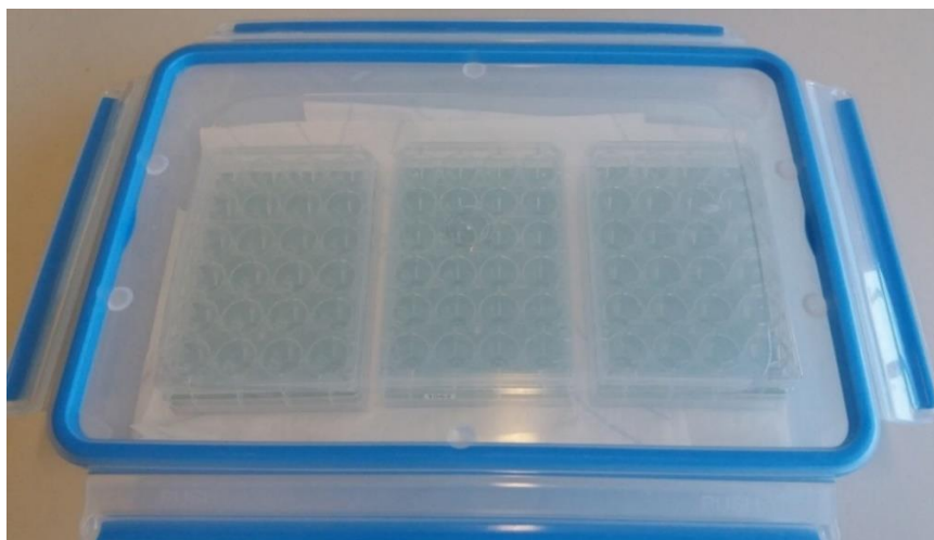
Fig. 4: Exemplary storage box with moistened paper towel, holding 3 Multiwell-MEA plates.
