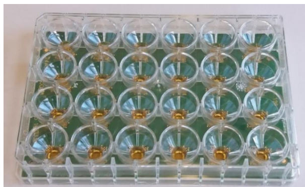
Fig. 1: 24-well glass Multiwell-MEA plate with PEDOT-coated gold electrodes.
