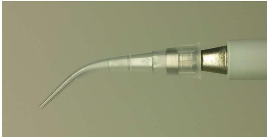
*Fig. 1: Kinked 10  $\mu$ l pipette. The tip was softened using a crème-brûle burner and a forceps.*
