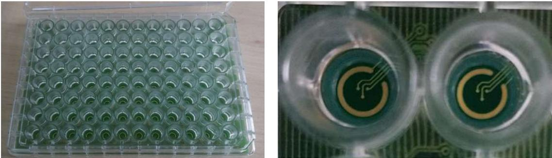
*Fig. 3: 96-well Multiwell plate. Left: Overview, right: Microscopic view into two wells. Note the three electrodes in the center of the well and the circular reference electrode. Cells ideally are only plated in the center without covering the reference electrode.*
